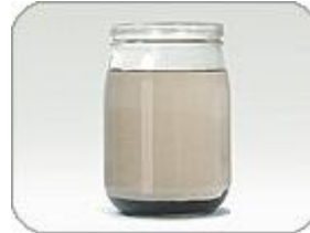
To demonstrate we put an example of black iron oxide sludge in to a container...
